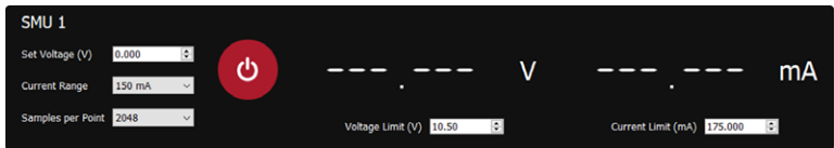
Figure 9.4. Control and output panel for the SMUs.
